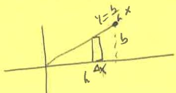
$$\text{Volume of slice } dV = \pi \left( \frac{b}{h} x \right)^2 \Delta x$$
